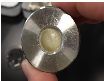
● 图3、某有机样品与KBr研磨压片
